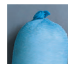
Socks filler expands and gels as liquid is absorbed
