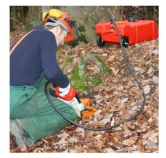
Explosion-suppressing insert (patent protected), hence no explosive atmosphere inside the container (Ex0 model only)
