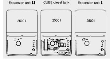
CUBE diesel filling station 7,500 L with expansion unit  ${\bf I}$  and  ${\bf II}$
