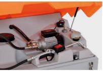
230 V electric gear pump 9 L/min at 12 bar with digital handheld flow meter for lubricants (cannot be calibrated\*)
